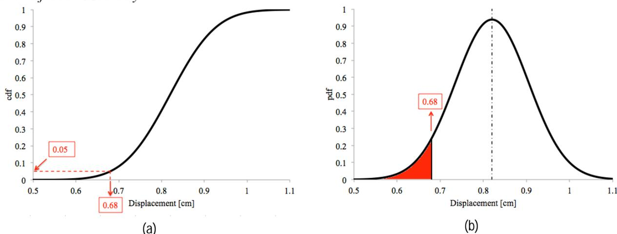
Figure 4.3: (a) Cumulative distribution function and (b) probability density function of the displacement capacity of an unreinforced masonry building class
