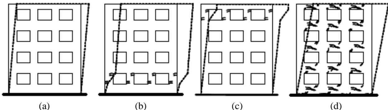
Figure 2.2: Deformed Shape for different limit states and in-plane failure modes (Restrepo-Velez and Magenes, 2004)
