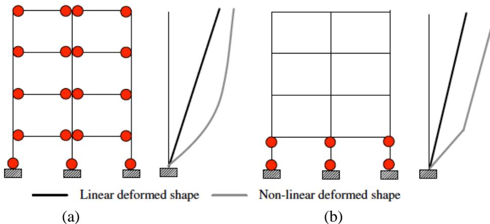
Figure 2.1: Response mechanisms for a frame and associated deformed shapes. (a) Beam Sway mechanism (b) Column Sway mechanism
