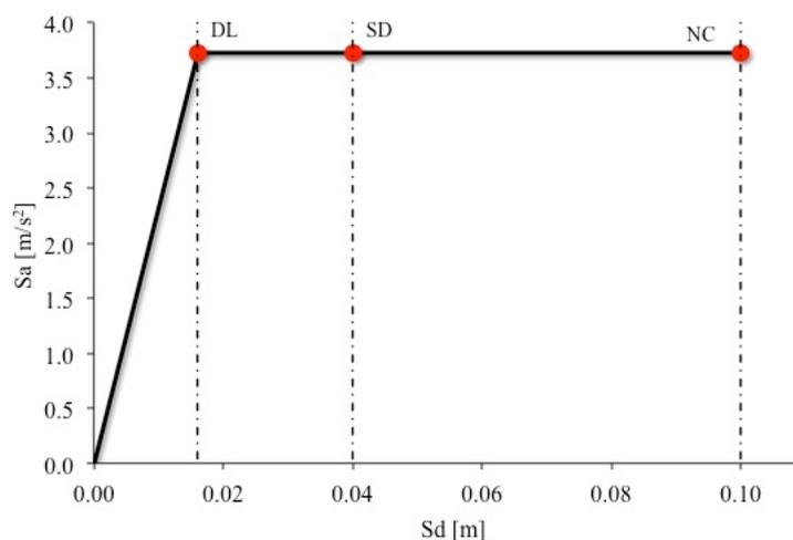
*Figure 1.1: Capacity Curve: Three Limit States*
