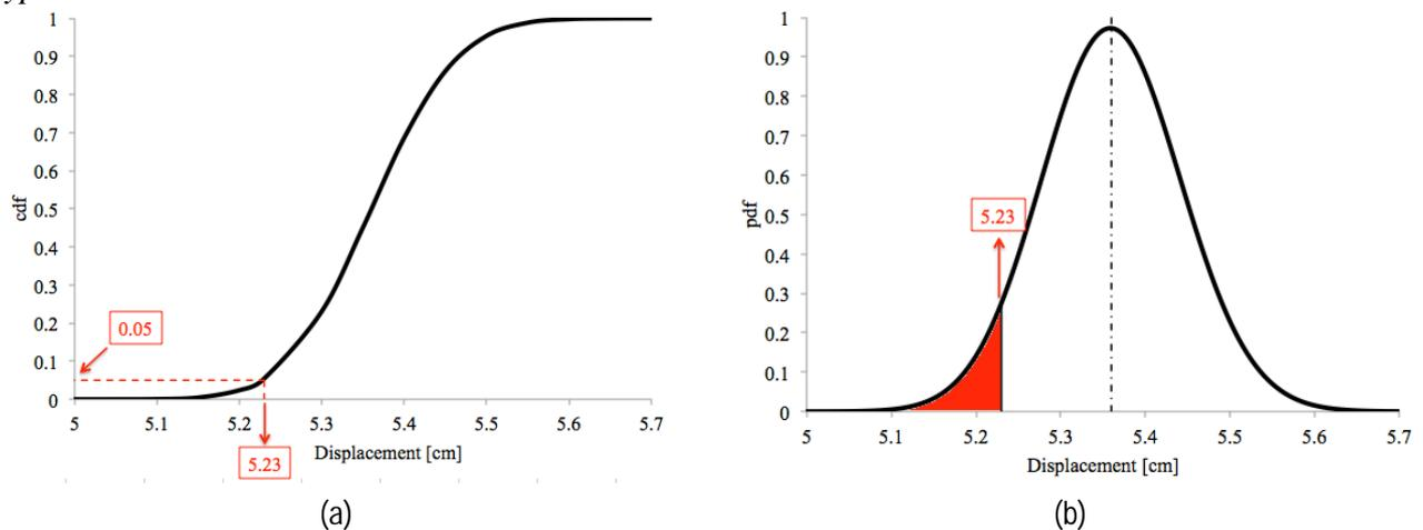
Figure 4.2: (a) Cumulative distribution function and (b) probability density function of the displacement capacity of a reinforced concrete building class (Steel Type 2)
