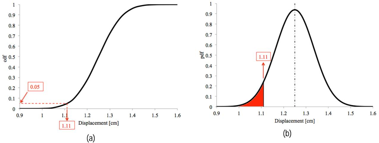
Figure 4.4: (a) Cumulative distribution function and (b) probability density function of the displacement capacity of reinforced masonry building class
