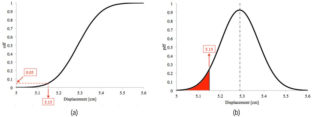
Figure 4.1: (a) Cumulative distribution function and (b) probability density function of the displacement capacity of a reinforced concrete building class (Steel Type 1)
